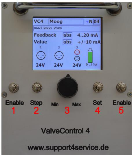
1. «Enable» button at the left – turns on/off the device output.
